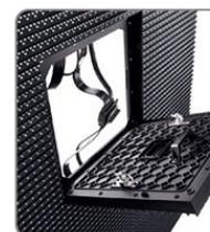
Disassemble cables, and take the module directly
