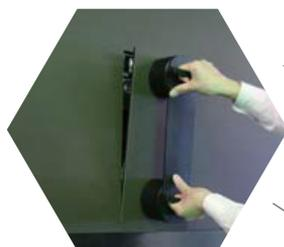
Keeping the tool against the module, rotate the magnetic discs clockwise until firmly secured.
